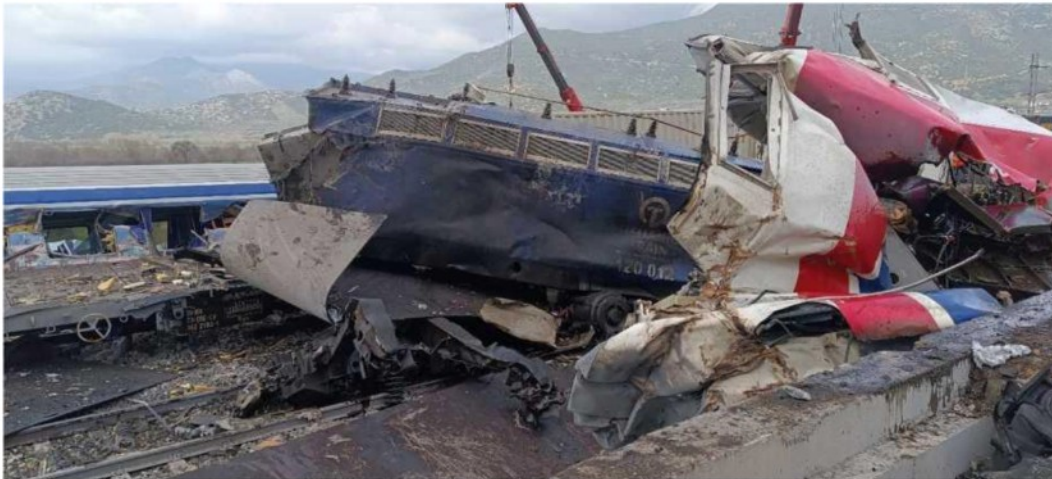
Figure 13. Locomotives 120-022 and 120-012 of the freight train 63503 after the accident. Front view, from the road.
