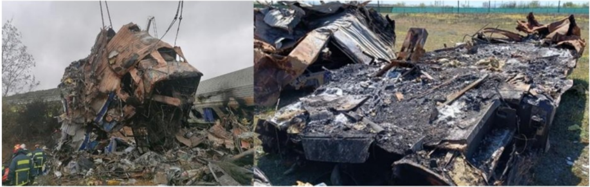
Figure 21. Remains of the Restaurant Car, on the left, S-shaped as found on-site, and on the right, its platform at Koulouri site.
