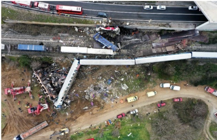
Figure 10. The end position of the 3 locomotives and some of the passengers coaches and freight wagons ( http://www.intime.gr/ ).
