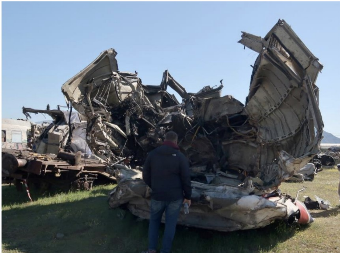
Figure 16. Front view of the locomotive 120-022, roof missing.
