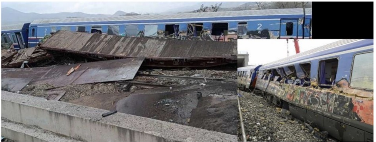
Figure 25. Linear impact of steel plates on the side of the coach B4.
